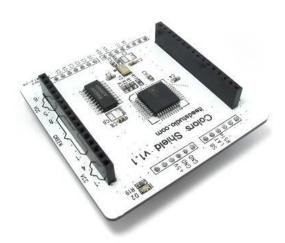
Colors shield is a magic RGB LED dot-matrix driver shield for Arduino or IFlat-32. Colors shield pairs the M54564 with a single <u>DM163</u> constant current driver. By using the DM163, the Colors shield gains three 8+6-bit channels of hardware PWM control of the LED's freeing up the MCU from having to implement it in software. This gives the ATmega more CPU bandwidth for performing other tasks.
