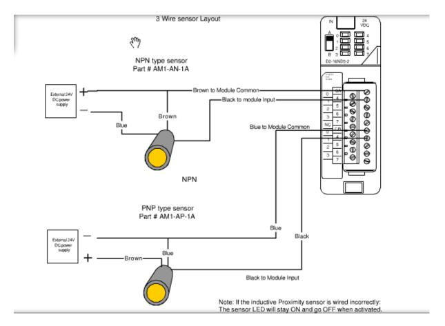
Connect the wires in the following order by finger twisting the bare ends together and covering the bare connection with the small wire nut. The black common should be connected to the power feed common of the control power system. The brown wire will tied to the power feed voltage, 12VDC to 36 VDC, depending on the type of switch. The blue wire will be connected to the device that is being electrically controlled, usually a small electric relay.
